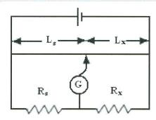
Q16 In a Wheatstone bridge experiment. The accuracy of the determination of the unknown resistor depends on:
